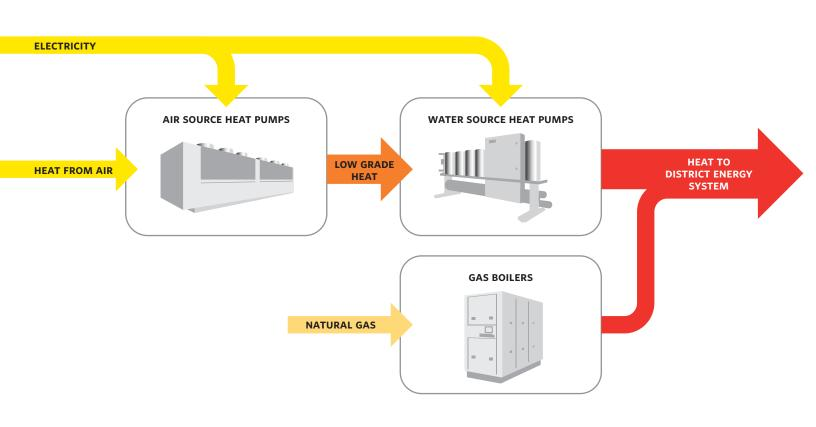
Example of two-stage air-source/water-source heat pump system with high-efficient boilers.
