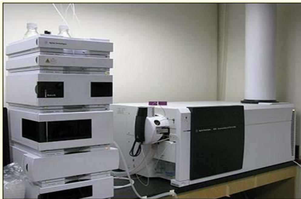
Figure 3.3 - Liquid Chromatography-Mass Spectrometry (LC/MS) system
