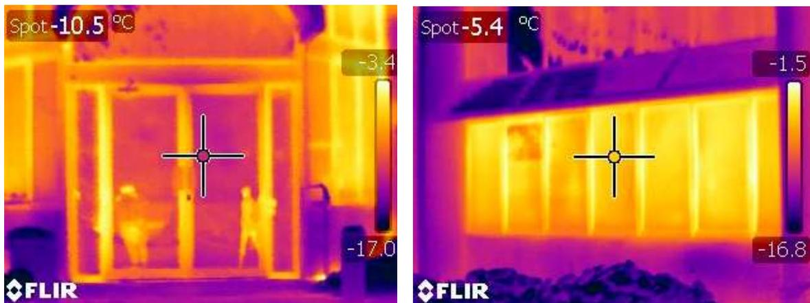
Figure 2.3: Main Building Entrance & Fenestration Thermographic Inspection
