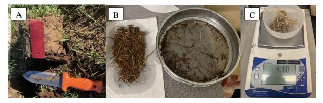
Figure 2.6: Method of root biomass collection: A) Field sample collection; B) Washing roots to remove dirt; C) Weighing washed and dried roots for final sample weight.
