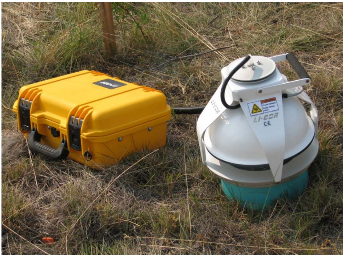
Figure 2.3. Automated Li-COR Soil CO 2 Flux System in operation
