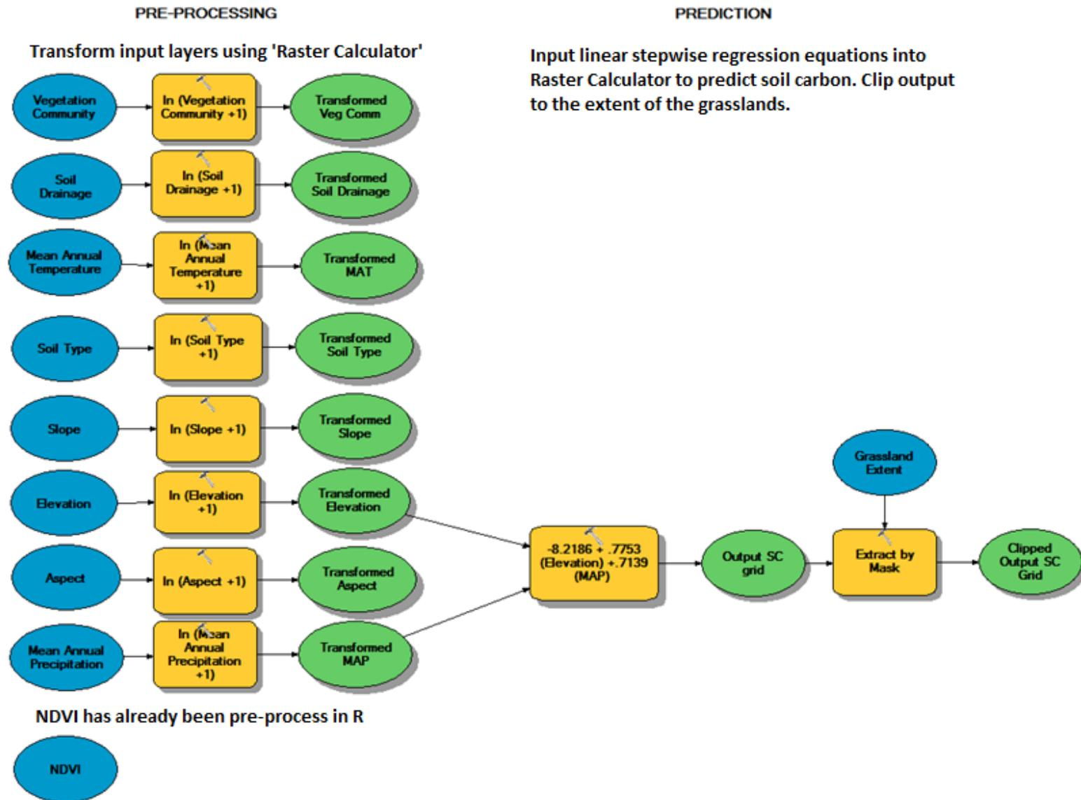
Figure 2.6: Example of model Builder flowchart for pre-processing data and creating predicted soil carbon grids with the stepwise regressions for 2013 soil carbon model of fenced systems
