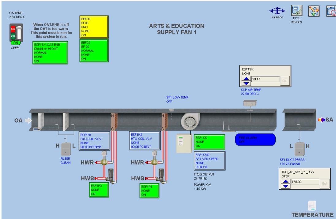
Figure 1: Makeup Air Unit SF-1 DDC Screen
