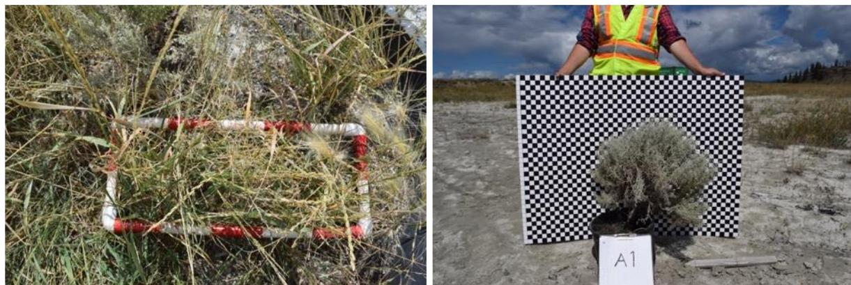
**Figure 3.8.** Assessing plant cover with a 0.25 m<sup>2</sup> quadrat (left) and measuring horizontal sagebrush canopy area with a custom 2-inch checkerboard (R) during 2016 data collection.
