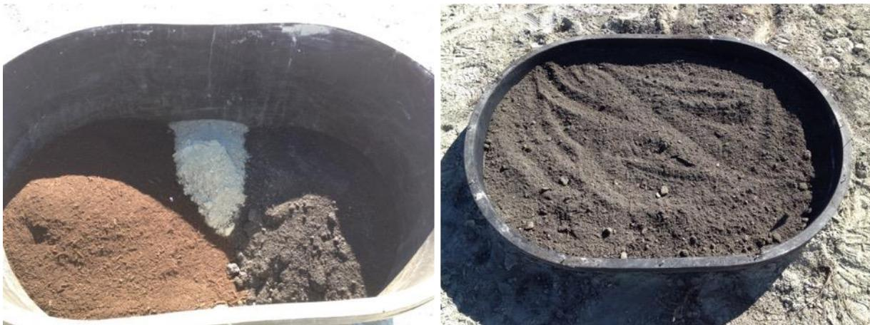
**Figure 3.4.** View of soil amendments and tailings prior to mixing (left) and amended study plot (right).
