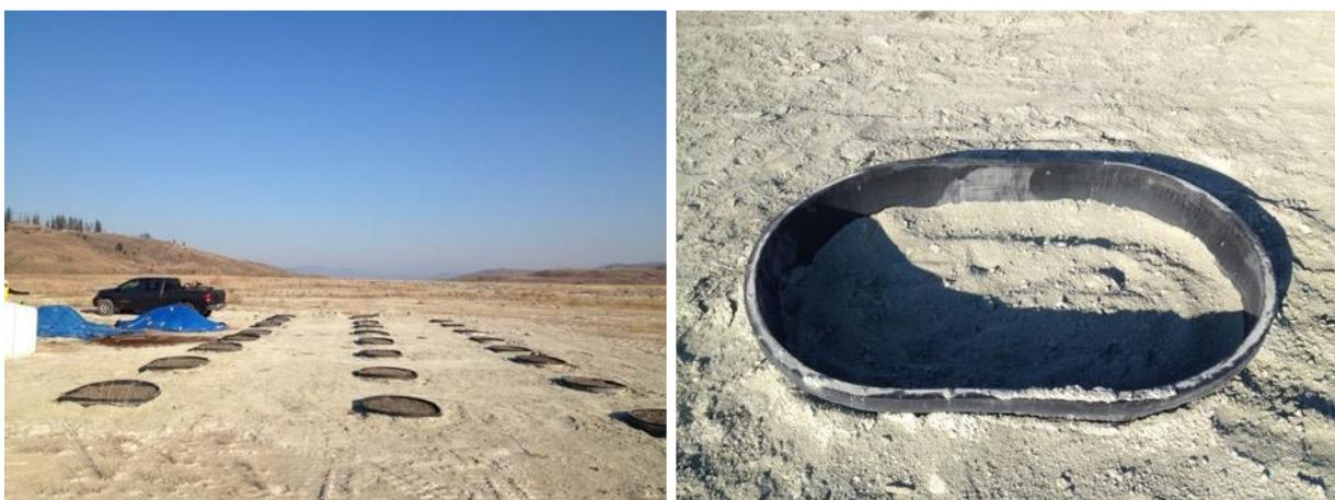
**Figure 3.2.** View of Historic Afton Tailings Storage Facility research plots (left) and individual plot containing unamended tailings (right).
