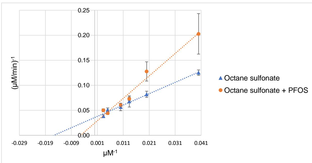
Figure 22. Lineweaver-Burk double reciprocal plot of SsuDH challenged with 6:2 FTSA (top) or octane sulfonate (bottom) in the presence (circle) or absence (triangle) of 200  $\mu\text{M}$  of PFOS. SsuDH was provided FMNH<sub>2</sub> by FreH. Error bars represent standard deviations (n=3).
