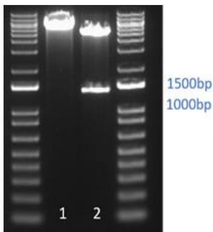
Figure 10. Restriction digestion analysis of pET281222. Restriction digestion was done with NcoI and HindIII; **1** digestion with HindIII **2** double digest. All DNA ladders are the 1 Kb Plus DNA Ladder (Invitrogen, Carlsbad, CA). Amplicons of the gene encoding ISGA 1222 are 1346 bp.
