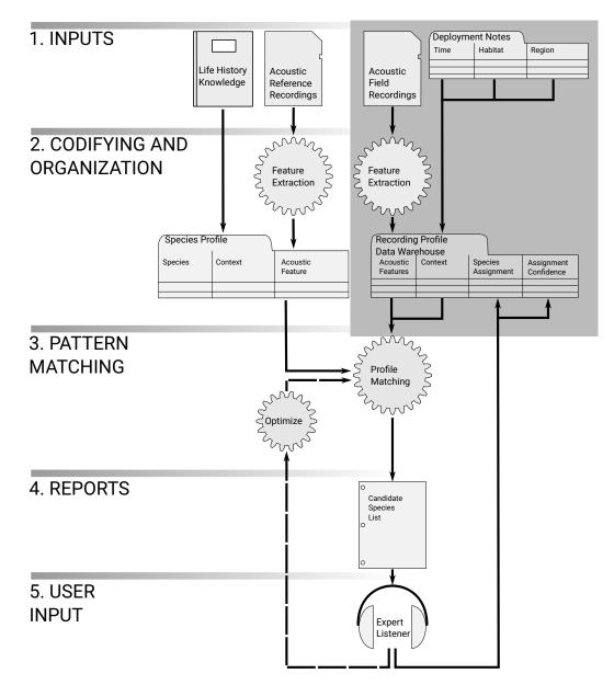
Figure 2.1: Components of a Decision Support System proposed to facilitate species identification by humans from bioacoustic recordings. The grey box indicates the focus of this research which was the creation of a data warehouse for bioacoustic data.
