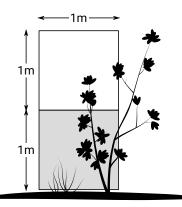
Figure 3.4: Sketch of a horizontal cover board in use. An estimate is made of how much each of the top and bottom squares are obscured by vegetation. In this example the top square is approximately 10% obscured and the bottom square it approximately 30% obscured.
