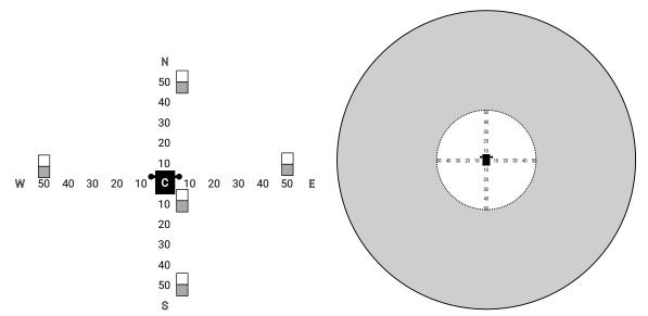
(a) Pattern at which water depths were measured around an ARU. Numbers indicate the distance in meters from the central point "C", where the ARU is placed.
