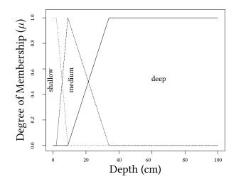
Figure 3.9: Membership functions for un-transformed water depths
