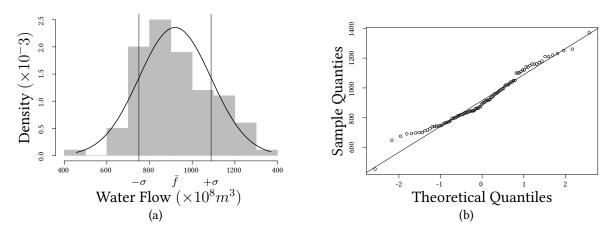
Figure 2.8: Distribution of water flow data used to derive fuzzy membership sets. The Q–Q plot shows that the distribution is approximately normal.
