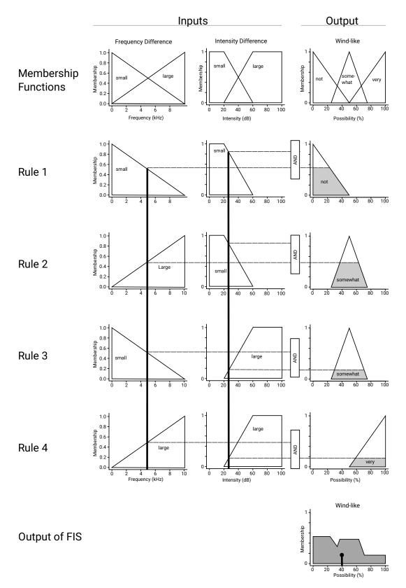
Figure 2.7: A fuzzy inference system to categorize acoustic signals as wind–sound. Two parameters of the four used by Towsey et al. (2012) are shown. An example is shown with input values: frequency difference = 4.691 kHz, intensity difference = 26.2 dB. Output: wind–like = 39.4%.
