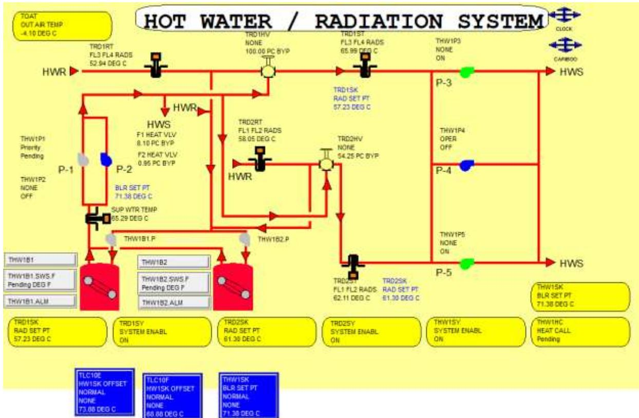
Figure 2.4: Hot water Radiation System – DDC Controls Graphics
