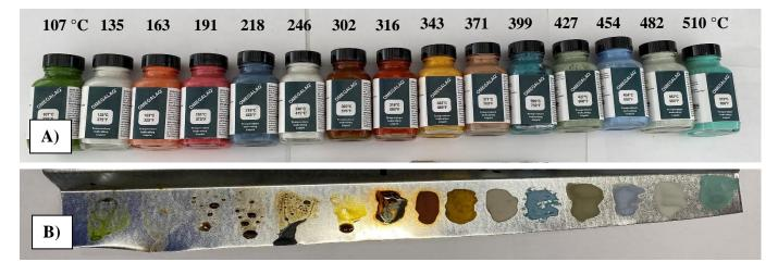
Figure 3.5. Omegalaq<sup>TM</sup> temperature sensitive paints applied at gradations of approximately 30 °C used to quantify fire temperature. A) Omegalaq<sup>TM</sup> paints from lowest to highest temperature. B) Example of paint change resulting from heat exposure in a lab setting.
