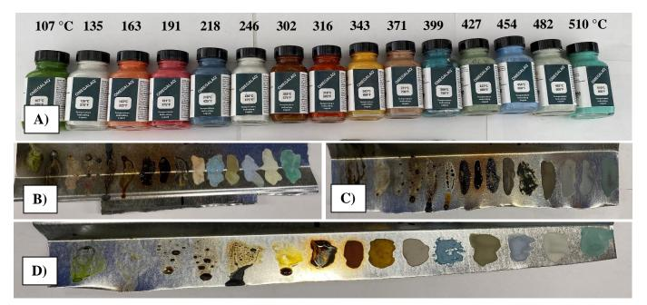
Figure 4.5. Omegalaq<sup>TM</sup> temperature sensitive paints applied at gradations of approximately 30 °C used to quantify fire temperature. A) Omegalaq<sup>TM</sup> paints from lowest to highest temperature. B) High severity burn analyzed at approximately 343 °C. C) Moderate severity burn analyzed at approximately 343 °C. D) Low severity burn analyzed at approximately 302 °C.
