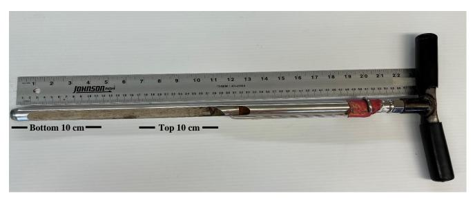
Figure 4.6. An intact soil core extracted from a mesocosm unit. The top 10 cm and bottom 10 cm was separated and used for soil analyses.
