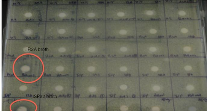
**Figure 6:** Primary screening of the 16 cave strains against *M. luteus*. The RA003 isolate showed antimicrobial activity against *M. luteus* when cultured in R<sub>2</sub>A and ISP#2 broth. The diameters of the zones were measured using sliding calipers.
