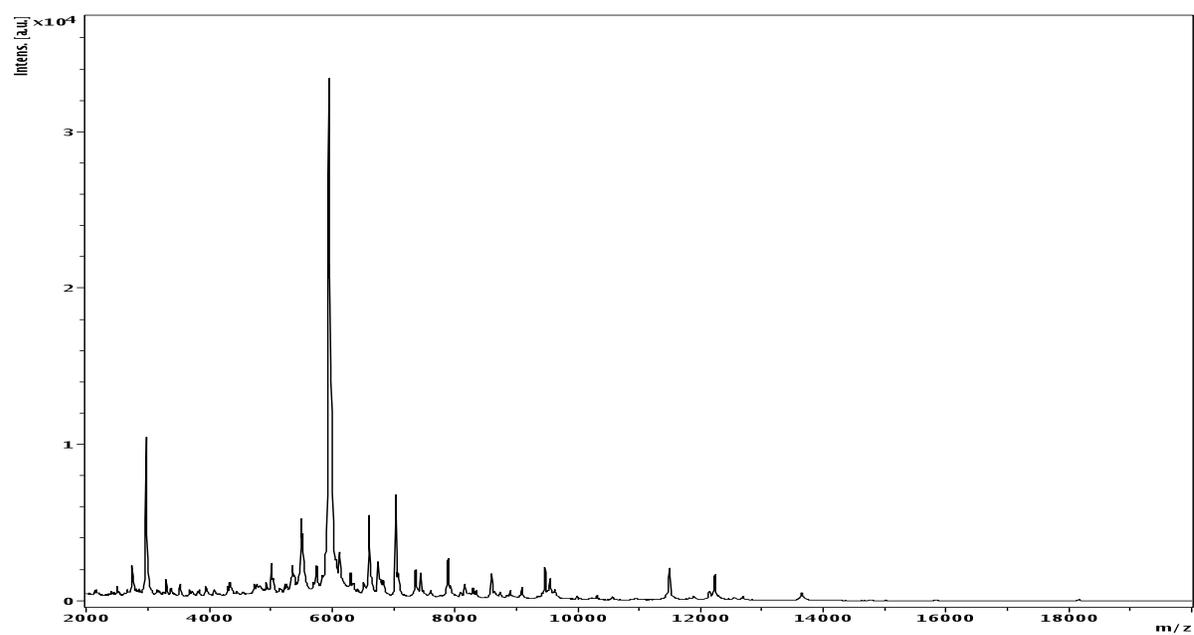
**Figure 25:** MALDI-TOF MS spectra for the RA004 isolate
