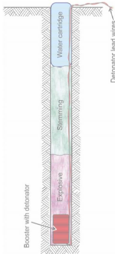
Figure 2.4 Blasting with Water Cartridges<sup>[8]</sup>
