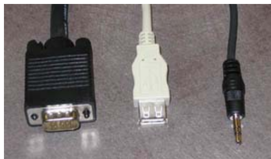
Laptop PC VGA, USB extension, and Audio connectors
