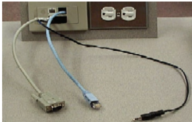
Laptop PC VGA, Network/LAN, and Audio connectors
